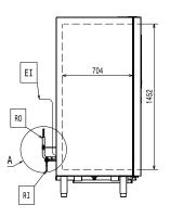
Electrical inlet (power) RO Refrigerant Outlet
